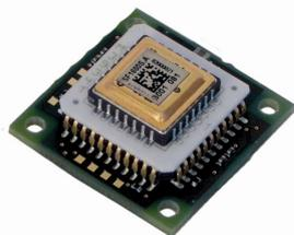
The SiFlex™ SF1600S.A and SF1600SN.a products combine a MEMS capacitive accelerometer, based on a bulk micro-machined silicon element in a ceramic package attached through an interconnect board to a custom mixed-signal ASIC to enable analog closed-loop force-feedback operation of the accelerometer. The multi-chip module (MCM) assembly is mounted to a printed circuit board consisting of power conditioning electronics employing linear regulators, output amplifiers and other support electronics.
